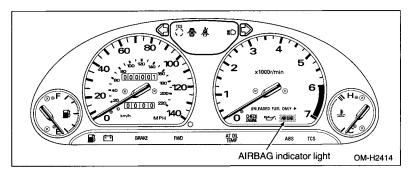
A diagnostic system continually monitors the readiness of the SRS AIR-BAG while the vehicle is being driven. The AIRBAG indicator light will show normal system operation by lighting for about 8 seconds when the ignition key is first turned to the "ON" position and then turning off.
