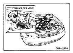
2. Find the Pressure Hold Valve. It is located inside the engine compartment under the brake fluid reservoir (big yellow cap).
