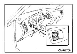
To turn off the TCS, push this switch while the engine is running. The indicator light on the switch will come on when the TCS is inactive. In this
