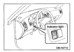
The TCS OFF indicator light comes on when the ignition switch is turned to the "ON" position and goes out within a few seconds after the engine starts. If the light does not come on when the ignition switch is turned "ON" and does not go out within a minute after the engine starts, it may indicate that TCS is not working properly. Contact your nearest SUBARU dealer immediately.
