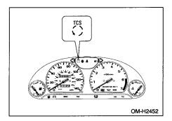
If the TCS indicator light comes on when driving, it indicate that the TCS is in operation.
