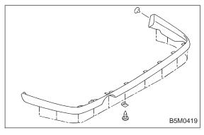
4) Remove roof spoiler mounting nuts.
