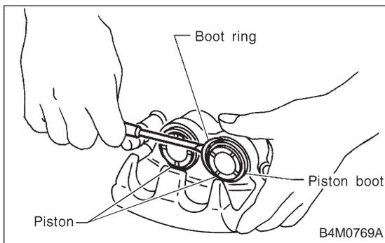
2) Using a standard screwdriver, remove boot ring from piston.
