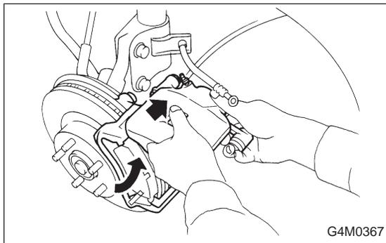
3) Raise caliper body and move it toward vehicle center to separate it from support.
