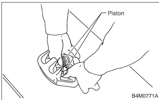
4) Insert piston into cylinder.
