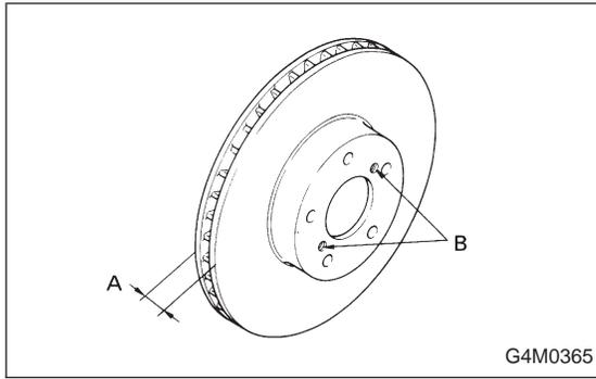
3) Measure disc rotor thickness.
