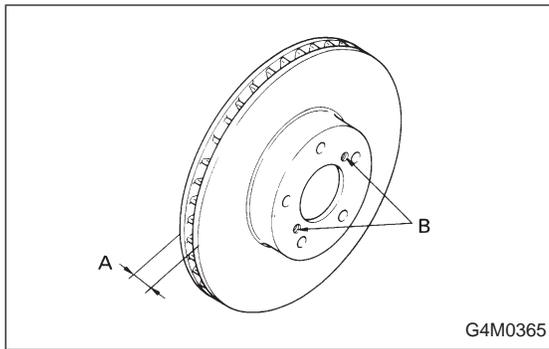
5) Remove disc rotor from hub.
