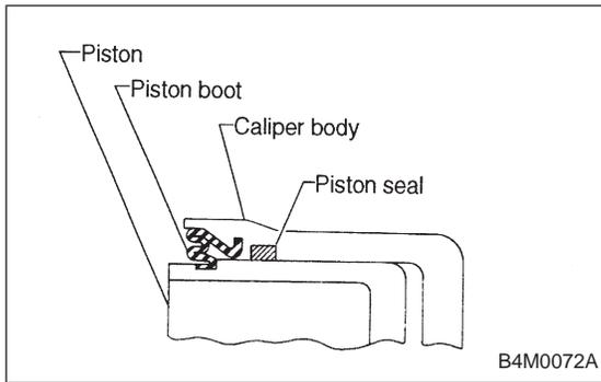
6) Position boot in grooves on cylinder and piston.
