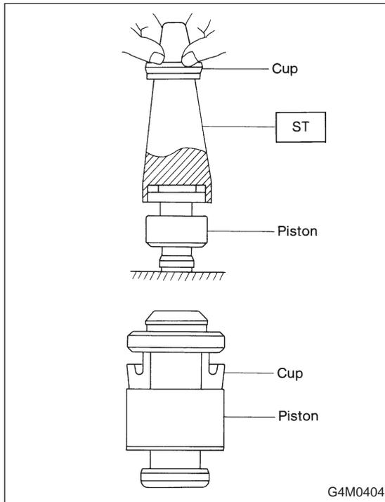
(1) When installing the cup, use ST, apply brake fluid to the frictional surface for smooth installation and pay attention to cup direction.
