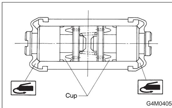
2) Apply rubber grease to the boot inside as shown in Figure.
