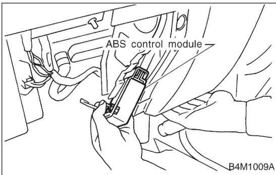
11) While holding the lower part of instrument panel rearward 5 cm (1.97 in) remove the ABSCM.
