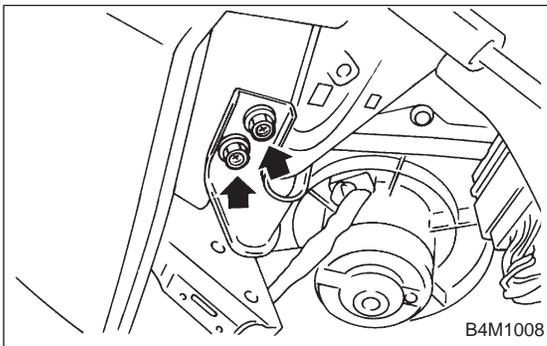
10) Remove two ABSCM lower mounting bolts from the lower part of the instrument panel.
