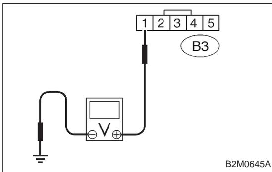
**10B3 CHECK POWER SUPPLY TO MASS AIR FLOW SENSOR.**
