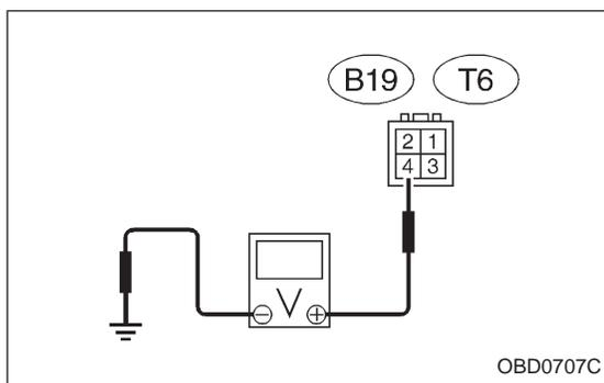
**10M4 CHECK HARNESS BETWEEN REAR OXYGEN SENSOR AND ECM CONNECTOR.**
