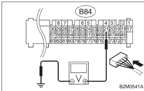
**10G2 CHECK INPUT SIGNAL FOR ECM. (USING VOLTAGE METER AND SUBARU SELECT MONITOR.)**
