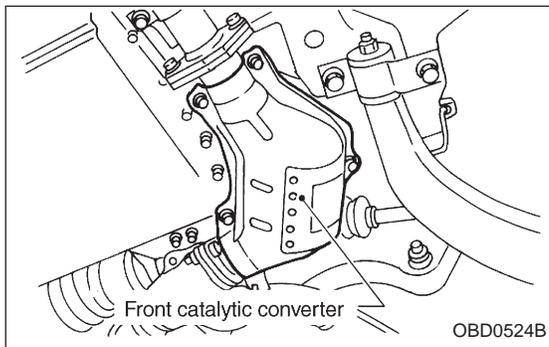
2) Remove front catalytic converter.
