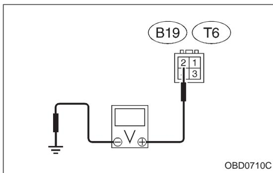
**1004****CHECK POWER SUPPLY TO REAR OXYGEN SENSOR.**
