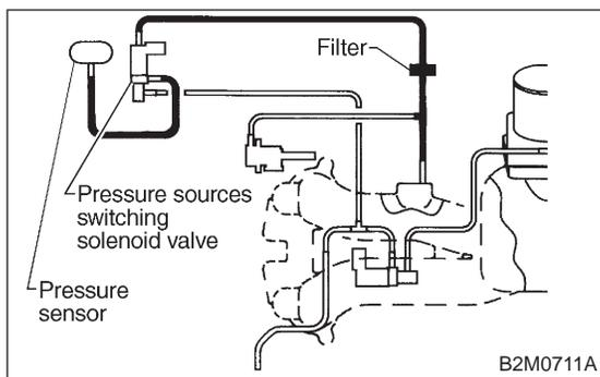
**10E3****CHECK VACUUM HOSE.****CHECK** : *Is there a fault in vacuum hose?***NOTE:**
