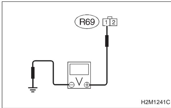
**10AJ5****CHECK POWER SUPPLY TO VENT CONTROL SOLENOID VALVE.**
