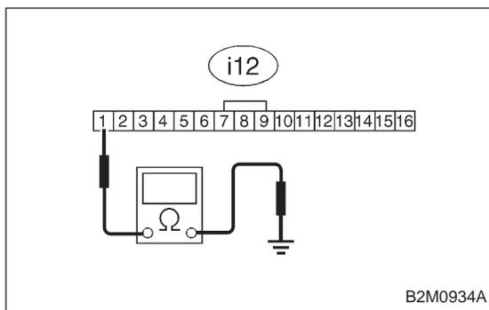
4) Measure resistance of harness between combination meter connector and chassis ground.
