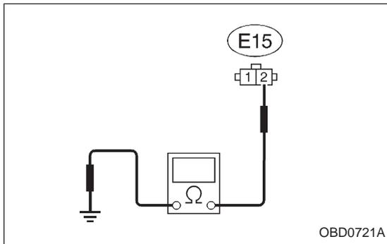
**CHECK** : **Connector & terminal (E15) No. 2 — Engine ground: Is the resistance less than 5 Ω?**
