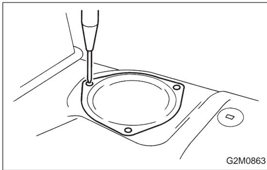
5) Remove service hole cover located on the left rear of trunk compartment floor (Sedan) or luggage compartment floor (Wagon).
