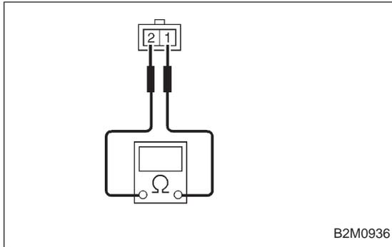
2) Disconnect connector from fuel sub meter unit.
