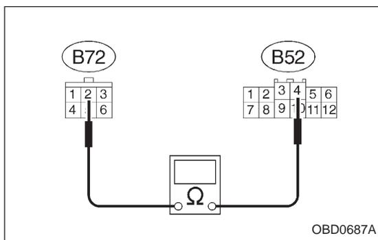
6) Measure resistance of harness between sub fan relay 1 (with A/C models) or main fan relay (without A/C models) and ignition switch connector.
