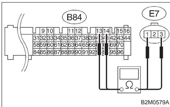
**10AN5 CHECK HARNESS BETWEEN ECM AND IDLE AIR CONTROL SOLENOID VALVE CONNECTOR.**
