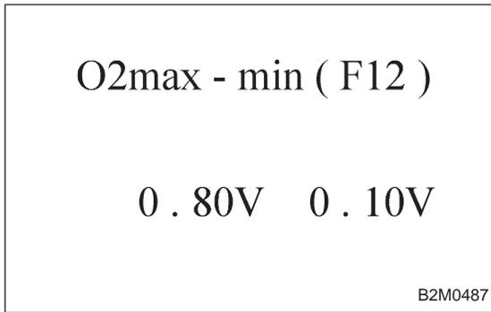
5) Read data on Subaru Select Monitor or the OBD-II general scan tool.
