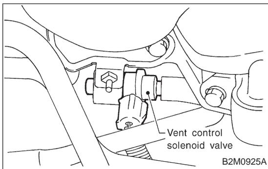
**CHECK** : *Does vent control solenoid valve produce operating sound?*
