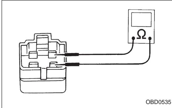
**10BQ3 CHECK MAIN FAN RELAY 1, SUB FAN RELAY 1 AND MAIN FAN RELAY.**
