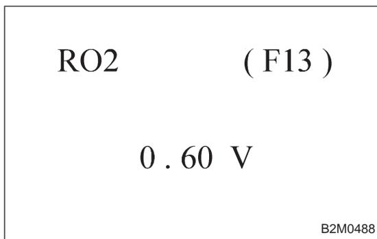
**CHECK** : *Is the value fixed between 0.2 and 0.4 V in function mode F13?*
