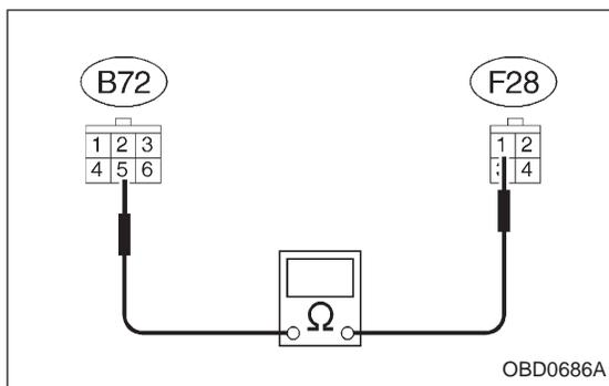
5) Measure resistance of harness between main fan relay 1 and ignition switch connector.
