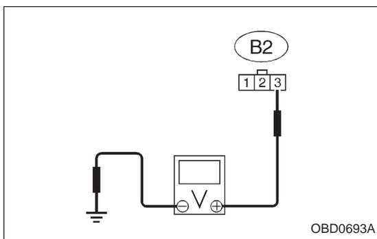
**10D3 CHECK HARNESS BETWEEN ECM AND PRESSURE SENSOR CONNECTOR.**
