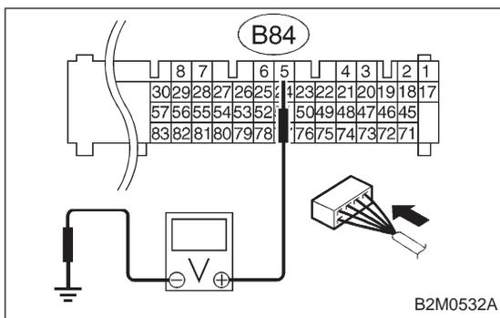
**10B2 CHECK INPUT SIGNAL FOR ECM. (USING VOLTAGE METER AND SUBARU SELECT MONITOR.)**
