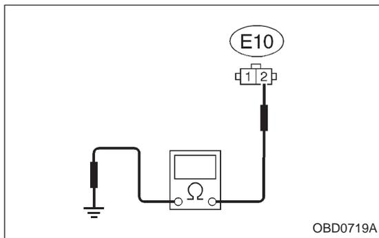
**CHECK** : **Connector & terminal (E10) No. 2 — Engine ground: Is the resistance less than 5 Ω?**
