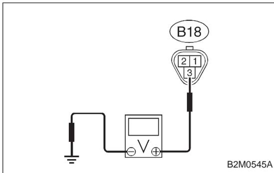
**10J3    CHECK HARNESS BETWEEN FRONT OXYGEN SENSOR AND ECM CONNECTOR.**
