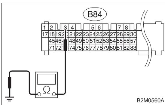
**CHECK** : **Connector & terminal (B84) No. 3 — Chassis ground: Is the resistance less than 400 kΩ?**
