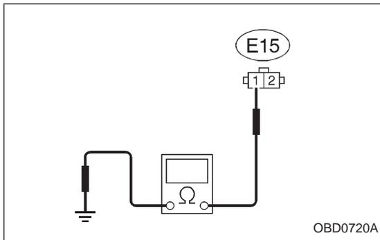
**CHECK** : **Connector & terminal (E15) No. 1 — Engine ground: Is the resistance less than 10 Ω?**
