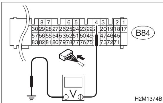
2) Measure voltage between ECM and chassis ground.
