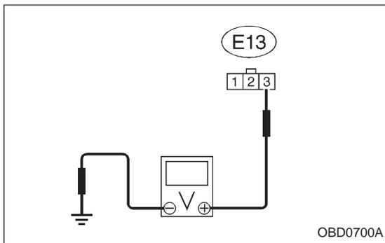
**10G3 CHECK HARNESS BETWEEN ECM AND THROTTLE POSITION SENSOR CONNECTOR.**
