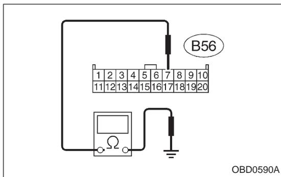
3) Measure resistance of harness between TCM and chassis ground.
