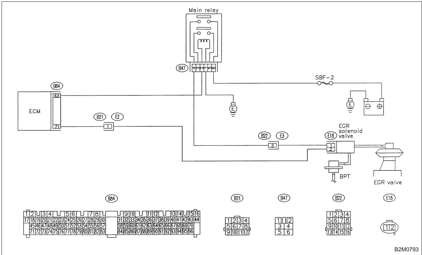
**10AE1 CHECK TRANSMISSION TYPE.****CHECK** : *Is transmission type AT?***YES** : Go to step 10AE2.**NO** : Check AT/MT identification circuit. <Ref. to 2-7 [T10BW0].>
