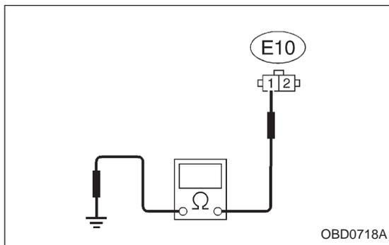
**CHECK** : **Connector & terminal (E10) No. 1 — Engine ground: Is the resistance less than 10 Ω?**
