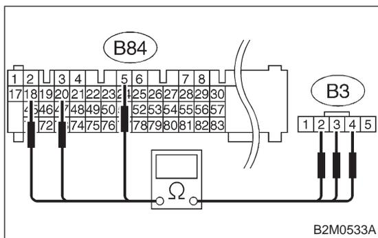
**10B4****CHECK HARNESS BETWEEN ECM AND MASS AIR FLOW SENSOR CONNECTOR.**
