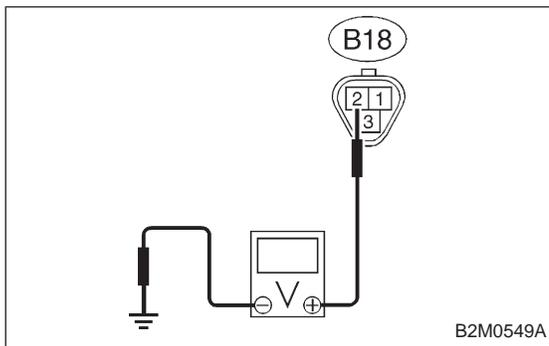
**10L4 CHECK POWER SUPPLY TO FRONT OXYGEN SENSOR.**
