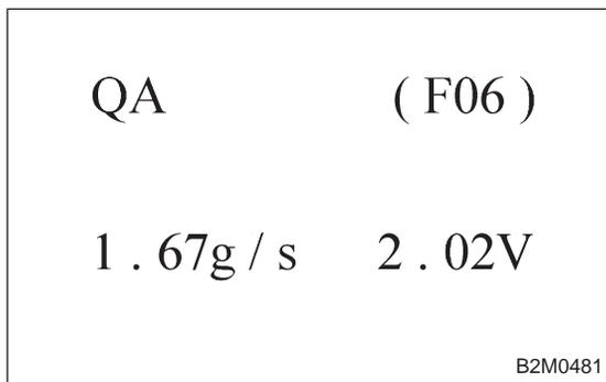
**CHECK** : *Is the value less than 1.3 g/sec or 0.3 V in function mode F06?*
