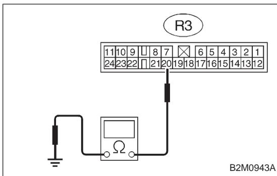
12) Separate rear wiring harness connector (R3) and bulkhead wiring harness connector (B99).
