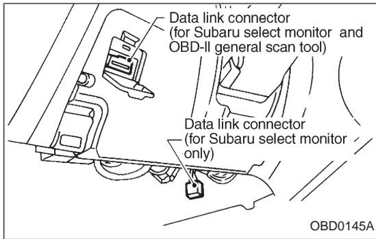
**10G1**      **CONNECT SUBARU SELECT MONITOR OR THE OBD-II GENERAL SCAN TOOL, AND READ DATA.**
