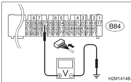
3) Measure voltage between ECM connector and chassis ground.
