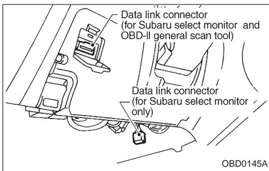
**10D1**      **CONNECT SUBARU SELECT MONITOR OR THE OBD-II GENERAL SCAN TOOL, AND READ DATA.**
