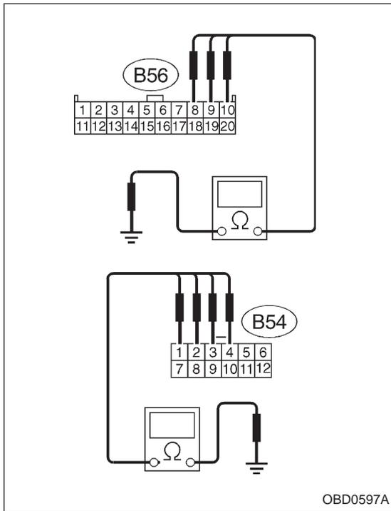
4) Measure resistance of harness between TCM and chassis ground.
