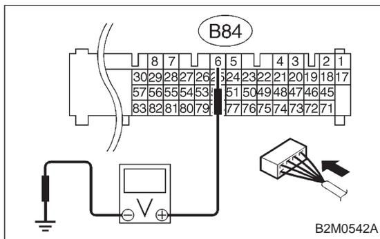
2) Measure voltage between ECM connector and chassis ground.
