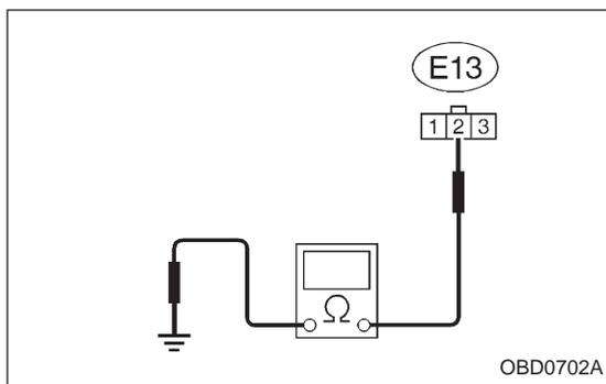
7) Measure resistance of harness between throttle position sensor connector and engine ground.
