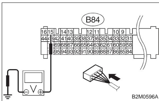
**10BL2 CHECK HARNESS BETWEEN ECM AND PRESSURE SOURCES SWITCHING SOLENOID VALVE CONNECTOR.**
