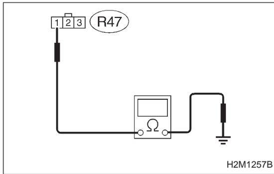
11) Measure resistance of harness between fuel tank pressure sensor connector and chassis ground.
