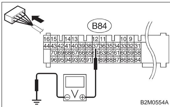
**1003 CHECK OUTPUT SIGNAL FROM ECM. (USING VOLTAGE METER.)**
