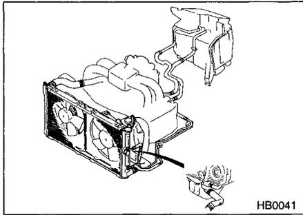
Your vehicle employs an electric cooling fan which is thermostatically controlled to operate when the engine coolant reaches a specific temperature.
