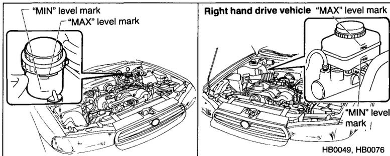
Check the fluid level on the outside of the reservoir. If the level is below "MIN", add the recommended brake fluid to "MAX".
