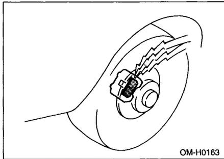
The front disc brakes and the right side rear disc brake have audible wear indicators on the brake pads. If the brake pads wear close to their service limit, the wear indicator makes a very audible scraping noise when the brake pedal is applied.
