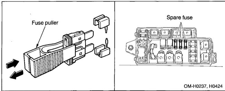
4. Pull out the fuse with the fuse puller provided in the interior fuse box cover.
