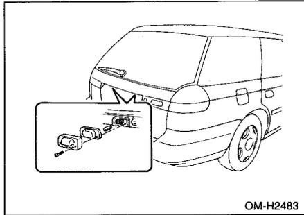
1. Remove the mounting screws using a phillips screwdriver.
