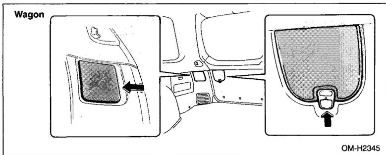
1. Unlatch the rear combination light cover by pulling the knob. Open the cover up.
