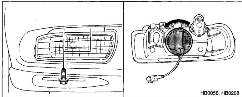
1. Remove the front fog light assembly by removing the two bolts.
