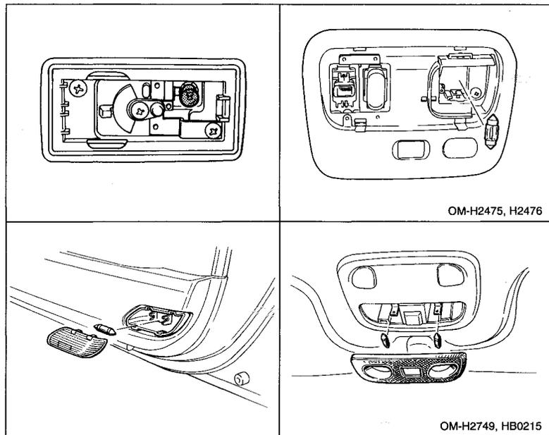
1. Remove the lens by prying the edge of the lens with a regular screwdriver.
