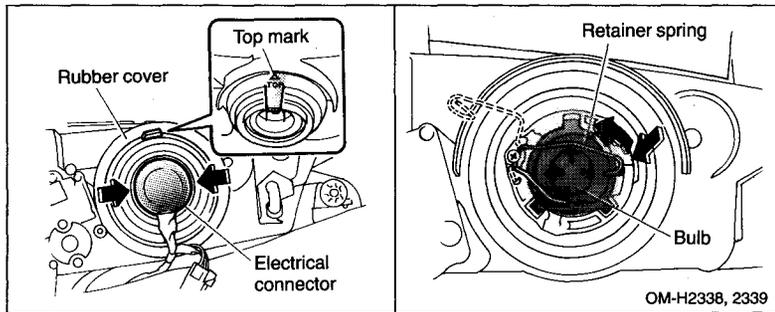
1. Disconnect the electrical connector, then remove the rubber cover.
