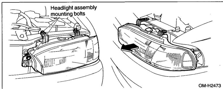
2. Remove the three headlight assembly mounting bolts then move the headlight assembly forward until it pops out from the fender.
