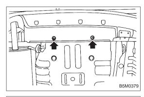
3) Remove two clips from lower center of bumper.
