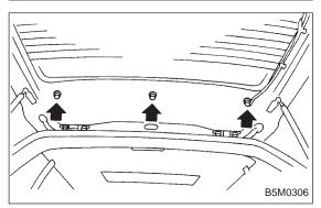
4) Remove roof spoiler mounting nuts.
