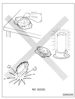
4) Do not drop the airbag modulator parts, subject it to high temperatures over 90°C (194°F), or apply oil, grease, or water to it; otherwise, the internal parts may be damaged and its reliability greatly lowered.
