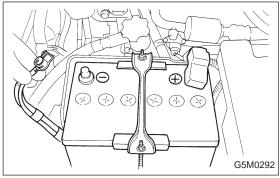
2) When servicing, be sure to turn the ignition switch off, disconnect the negative (-) battery terminal then the positive (+) terminal in advance, and wait for more than 20 seconds before starting work.
