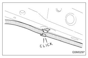
6) Install the wire harness securely with the specified clips so as to avoid interference or jamming with other parts.
