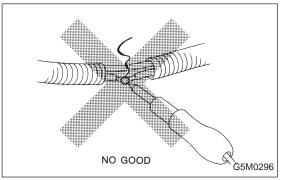
5) If any damage or open is found on the SRS airbag system wire harness, do not attempt to repair using soldering, etc. Be sure to replace the faulty harness with a new genuine part.
