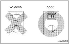
3) When checking the system, be sure to use a digital circuit tester. Use of an analog circuit tester may cause the airbag to activate erroneously. Do not directly apply the tester probe to any connector terminal of the airbag. When checking, use a test harness.
