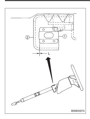
• Check to ensure that clearance between capsule ① (at steering column) and cutout portion of column bracket ② on steering column upper side is within specifications.
