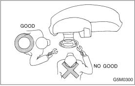
When removing and installing the airbag module (driver side and passenger side), the operator should stand, as much as possible, on the side of the airbag module.
