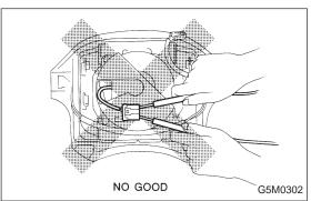
Do not check airbag module (driver side and passenger side) continuity with airbag removed from the vehicle body.
