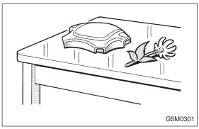
• After removal, the airbag module (driver side and passenger side) should be kept away from heat and light sources, and stored on a clean, flat surface to prevent from any damage to its lower structure.
