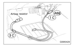
10) Turn ignition switch "OFF", disconnect battery ground cable, and wait 20 seconds. Remove lower cover panel and connect test harness C connector (1C) to (AB8) <Ref. to 5-4 [W1A0].> with airbag resistor attached to test harness C connector (3C).
