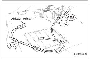
7) Turn ignition switch "OFF", disconnect battery ground cable, and wait 20 seconds. Connect passenger side airbag module connector (AB9) to (AB10). Connect battery ground cable and turn ignition switch "ON". Does airbag warning light go "OFF" after about 7 seconds and remain off for more than 30 seconds?
