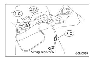
11) Turn ignition switch "OFF", disconnect battery ground cable, and wait 20 seconds. Disconnect passenger side airbag module connector (AB9) to (AB10). <Ref. to 5-5b [W3A2].>
