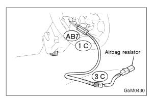
8) Turn ignition switch "OFF", disconnect battery ground cable, and wait 20 seconds. Connect connector (AB8) to (AB3). Remove driver side airbag module and connect test harness C connector (1C) to (AB7). <Ref. to 5-5b [W3A1].> Connect airbag resistor to test harness C connector (3C). Connect battery ground cable and turn ignition switch "ON". Does airbag warning light go "OFF" after about 7 seconds and remain off for more than 30 seconds? See "NOTE:".
