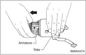
Installing armature to yoke
