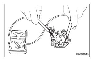
3) Insulation resistance of brush holder Be sure there is no continuity between brush holder and its plate.
