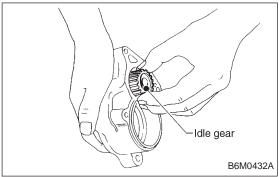
12) Remove idle gear from housing.
