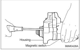
8) Remove screws securing magnetic switch to housing.
