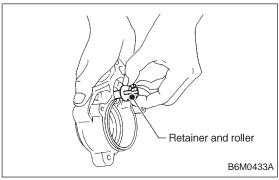
13) Remove retainer and roller from housing.
