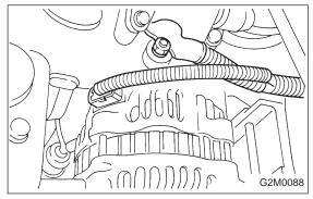
2) Disconnect connector and terminal from generator.
