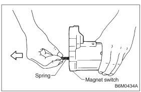
14) Remove coil spring from magnetic switch.
