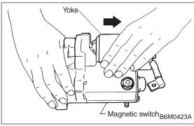
3) Remove yoke from magnetic switch.
