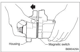
9) Remove housing from magnetic switch.
