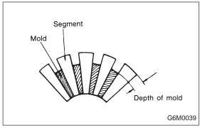
3) Depth of segment mold Check the depth of segment mold.
