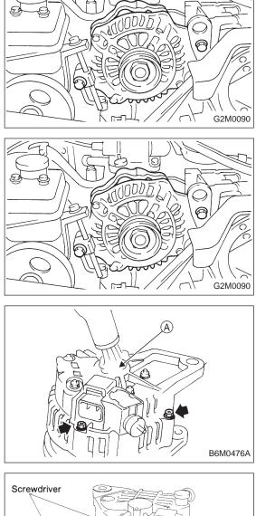
5) Remove bolts which install generator onto bracket.
