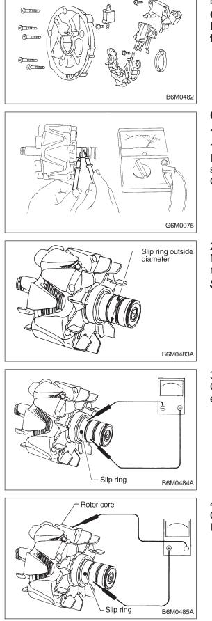
8) Remove bolts which secure IC regulator, diode and brush holder.
