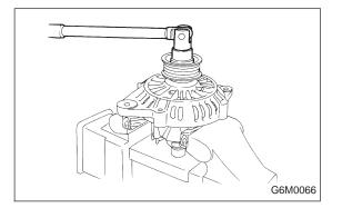
3) Hold rotor with a vise and remove pulley nut.
