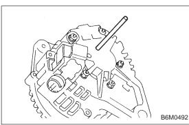
• When installing rear cover, heat portion (Å) to 50°C (122°F) with heater drier.
