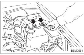
3) Remove washer tank mounting bolts.
