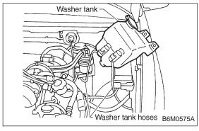
5) Move washer tank upward.
