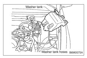
5) Move washer tank upward.
