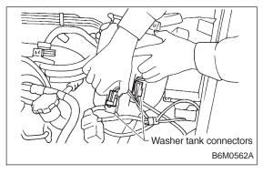
4) Disconnect washer tank connectors.
