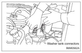
4) Disconnect washer tank connectors.
