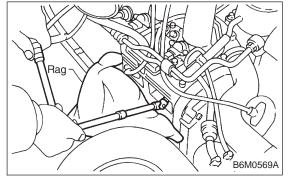
9) Set 4 extension and 5 ratchet in turn onto the connected tools in plug hole, and remove spark plug using them.
