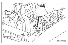
4) Remove spark plug with the spark plug socket.
