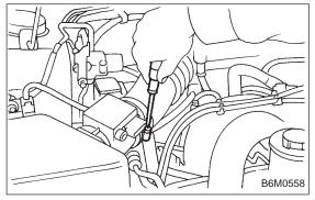
4) Loosen the clamp screw and separate air cleaner upper cover from air intake duct.
