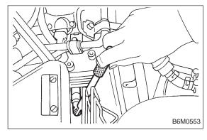
3) Remove spark plug with the spark plug socket.
