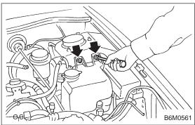
3) Remove washer tank mounting bolts.
