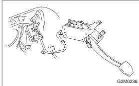
4) Depress clutch pedal to assure there is no abnormality in the clutch system.
