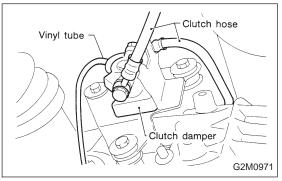
2) Slowly depress the clutch pedal and keep it depressed. Then open the air bleeder to discharge air together with the fluid
