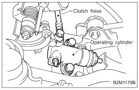
2) Remove clutch hose from operating cylinder.
