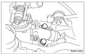
3) Remove operating cylinder from transmission.
