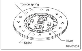
5) Worn spline, loose rivets and torsion spring failure Replace defective parts.
