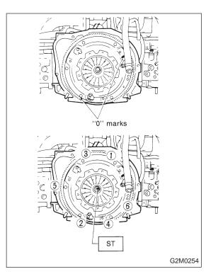
4) Install clutch cover on flywheel and tighten bolts to the specified torque.
