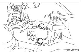
3) Remove operating cylinder from transmission.
