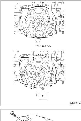
4) Install clutch cover on flywheel and tighten bolts to the specified torque.
