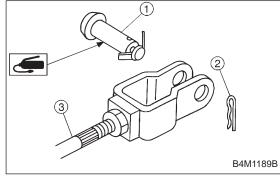
3) Connect push rod 3) of master cylinder to clutch pedal, and install clevis pin (1) and snap pin (2).
