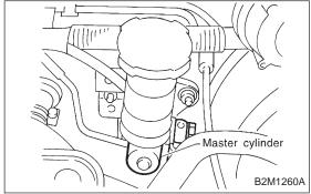
2) Remove clutch hose from master cylinder.
