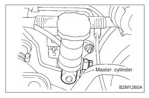
2) Install clutch hose to master cylinder.
