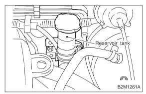
3) Remove master cylinder with reservoir tank.
