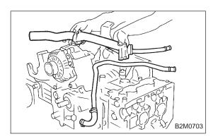
3) Install engine coolant pipe.
