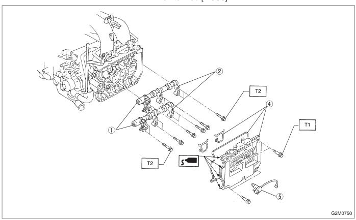
Tightening torque: N·m (kg-m, ft-lb) T1: 10±0.7 (1.0±0.07, 7.2±0.5) T2: 20±2 (2.0±0.2, 14.5±1.4) 2) Install camshaft sprockets, timing belt and related parts. <Ref. to 2-3b [W2C0].>
