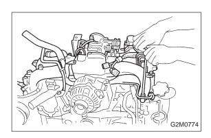
4) Install intake manifold.
