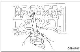
3) Measure inner diameter of valve lifter mating part on cylinder head.
