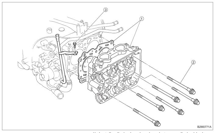
1) Install cylinder head and gaskets on cylinder block.
