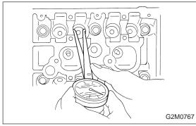
3) Measure inner diameter of bush on cylinder head.
