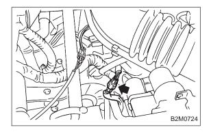
9) Connect front oxygen sensor connector.
