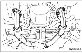
6) Remove bolts which hold front exhaust pipe onto cylinder heads.
