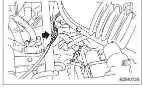
2) Disconnect rear oxygen sensor connector. (California 2200 cc model)
