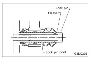
7) Apply a coat of specified grease to guide pin, outer surface, sleeve outer surface, cylinder inner surface, and boot grooves.
