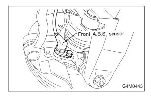
2) Temporarily install front ABS sensor on housing.
