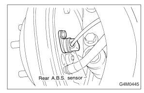
3) Remove rear ABS sensor from rear back plate.
