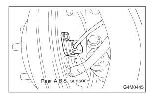
2) Temporarily install rear ABS sensor on back plate. **CAUTION:**
