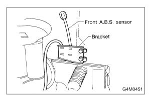
4) Install front ABS sensor on strut and wheel apron bracket.
