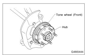
7) Remove tone wheel while removing hub from housing and hub assembly. <Ref. to 4-2 [W1B0].>
