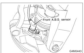
4) Remove bolts which secure front ABS sensor to housing, and remove front ABS sensor.
