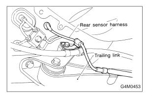
4) Install rear sensor harness on rear trailing link.
