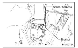
2) Remove bolts which secure sensor harness to strut.
