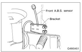
3) Remove bolts which secure sensor harness to body.
