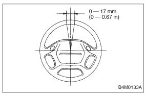
3) If steering wheel spokes are not horizontal when wheels are set in the straight ahead position, and error is more than 5° on the periphery of steering wheel, correctly re-install the steering wheel.
