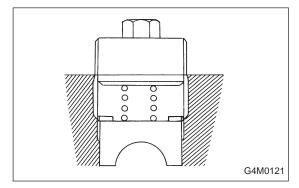
(4) Tighten adjusting screw by two threads.
