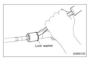
7) Bend lock washer using a chisel.
