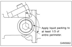
(5) Apply liquid packing to at least 1/3 of entire perimeter of adjusting screw thread.
