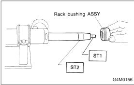
5) Fit ST1 and ST2 over the end of rack, and install rack bushing.
