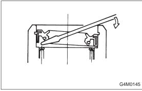
3) Pry off oil seal using screwdriver.
