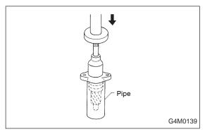
3) Draw out pinion and valve assembly from valve housing, as necessary, using pipe of I.D. 44 to 46 mm (1.73 to 1.81 in) and a press.
