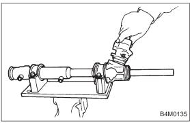
2) Install packing on valve assembly. Insert valve assembly into place while facing rack teeth toward pinion.
