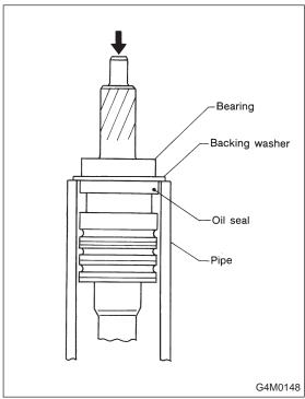
2) Press out bearing together with backing washer using pipe of I.D. 38.5 to 39.5 mm (1.516 to 1.555 in) and press.
