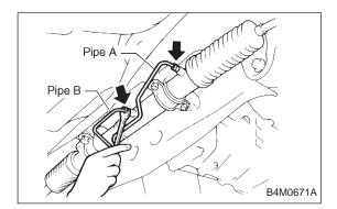
9) Connect pipes A and B to four pipe joints of gearbox. Connect upper pipe A first, and lower pipe B second.
