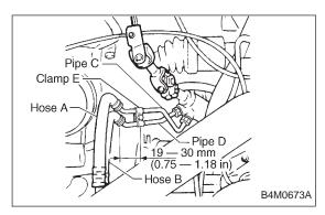
5) Temporarily connect pipes C and D to control valve of gearbox.
