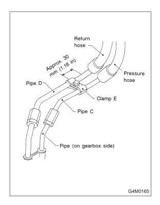
5) Temporarily connect pipes C and D to pipes (on the gearbox side).
