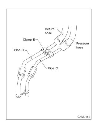
4) Remove clamp E from pipes C and D.
