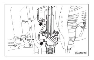
9) Connect pipes A and B to four pipe joints of gearbox. Connect upper pipe B first, and lower pipe A second.
