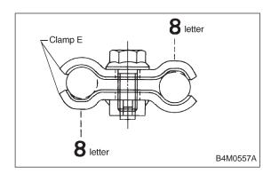
6) Temporarily install clamp E on pipes C and D.
