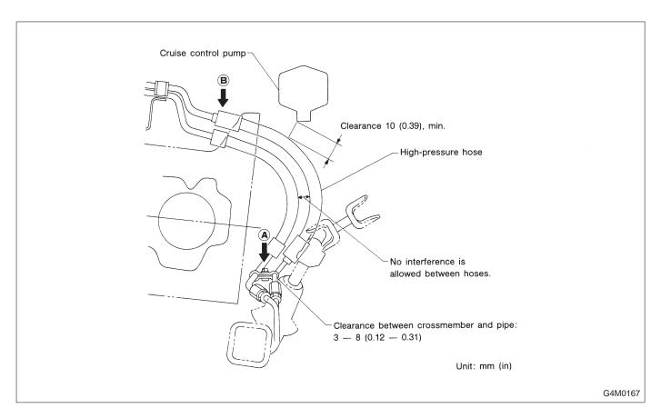
13) Finally check clearance between pipes and/or hoses, as shown above.
