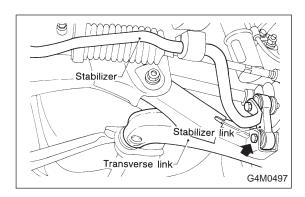
4) Connect stabilizer link to transverse link, and temporarily tighten bolts.
