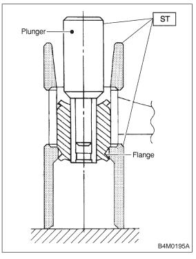
2) Press ST plunger until bushing flange protrudes beyond trailing link.
