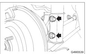
9) Remove bolts which secure rear strut to housing.
