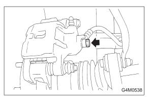
7) Models equipped with rear disc brakes: Remove union bolt from brake caliper. 8) Models equipped with rear drum brakes: Disconnect brake hose from brake pipe from strut, and disconnect brake pipe from dram brake.
