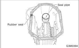
17) Install the rubber seal to the torque converter clutch case.
