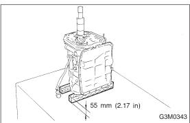
5) Place two wooden blocks on the workbench, and stand the transmission case with its rear end facing down.
