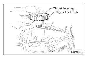
16) Take out the high clutch hub and the thrust bearing.
