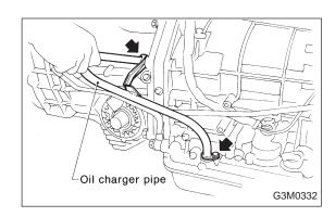
6) Install the oil charge pipe.
