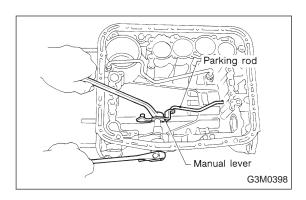
4) Assemble the manual lever and parking rod to the inside shaft, and secure with a nut.
