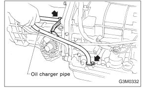
8) Remove the oil charger pipe, and remove the O-ring from the flange face. Attach the O-ring to the pipe.
