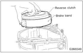
14) Remove the brake band and reverse clutch.
