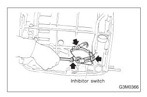
30) Remove the inhibitor switch.
