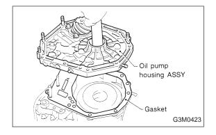
(3) Install both parts with dowel pins aligned. Make sure no clearance exists at the mating surface.
