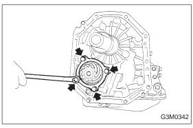
4) Loosen the taper roller bearing mounting bolts.
