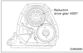
5) Install the reduction drive gear assembly.
