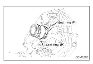
16) Apply vaseline to the groove on the oil pump cover, and install two (R) seal rings and two (H) seal rings.
