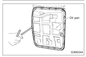
6) Remove the oil pan and gasket.
