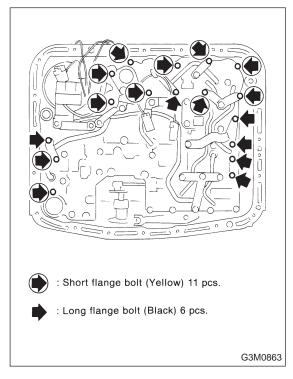
10) Remove the control valve body and the two brackets.
