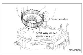
21) Take out the one-way clutch outer race and the thrust washer.
