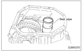
12) Install the seal pipe to the torque converter clutch case.
