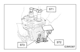
(7) Turn the drive pinion several rotations with ST1 and check to see if the backlash is within the standard value with ST2 and ST3.
