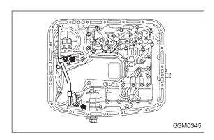
7) Remove the oil cooler outlet pipe.
