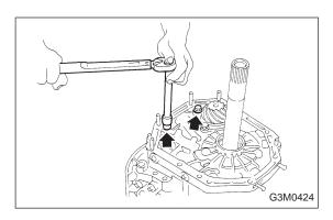
(4) Secure the housing with two nuts.
