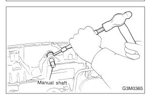
29) Remove the parking rod together with the manual lever. Then remove the manual shaft by pulling off the straight pin.
