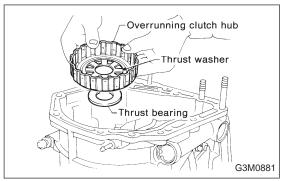
22) Take out the overrunning clutch hub, the thrust washer and the thrust bearing.
