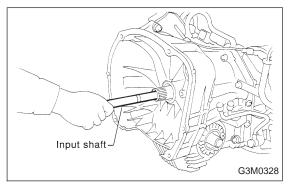
5) Remove the input shaft.
