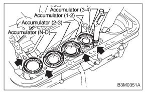
26) Apply compressed air from the operating pressure side, and take out accumulator (3-4), accumulator (1-2), accumulator (2-3), accumulator and spring (N-D).
