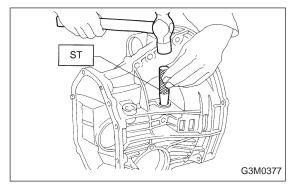
2) Install the washer and snap ring to the speedometer shaft with ST, and set the oil seal. Then force-fit the shaft to the torque converter clutch case.
