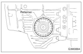
(5) Tighten the LH retainer until contact is felt while rotating the shaft. Then loosen the RH retainer. Keep tightening the LH retainer and loosening the RH retainer until the pinion shaft can no longer be turned. This is the "zero" state.
