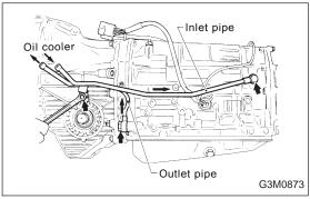
9) Remove the oil cooler inlet and outlet pipes.
