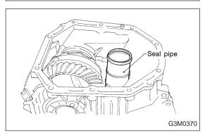
Remove the differential case assembly.
