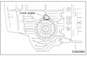
(6) After the "zero" state is established, back off the LH retainer 3 notches and secure it with the lock plate. Then back off the RH retainer and retighten until it stops. Repeat this procedure several times. Tighten the RH retainer 1-3/4 notches further. This sets the preload. Finally, secure the retainer with its lock plate.
