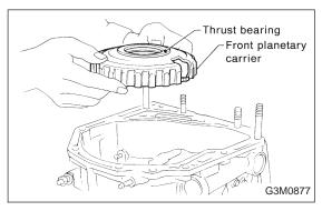
18) Take out the front planetary carrier and the thrust bearing.
