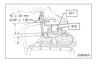
(2) Measure the distance " $\ell$ " from the transmission case mating surface to the reduction drive gear end surface with ST1 and ST2. (On FWD models, measure distance from end of case to end of bearing.)
