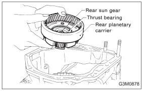
19) Take out the rear planetary carrier, rear sun gear and the thrust bearing.
