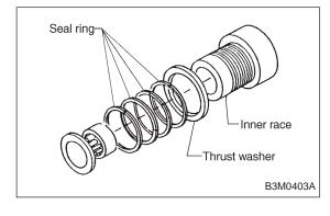
(2) Install four seal rings and thrust washer.
