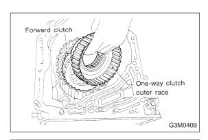
13) Install the one-way clutch outer race.
