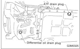
2) Remove the drain plug, and drain differential oil. Tighten the plug temporarily after draining.
