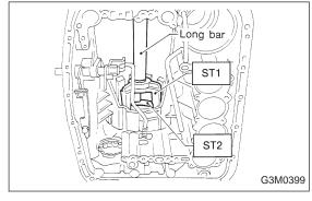
6) Install the lathe cut seal rings to the I.D./O.D. of the low and reverse piston. Then install the piston into the case with a press, ST1 and ST2.
