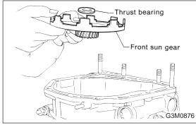
17) Take out the front sun gear and the thrust bearing.
