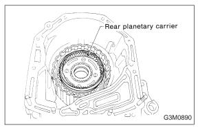
15) Install the rear planetary carrier.
