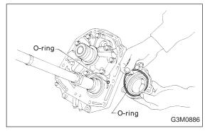
14) Attach the O-ring to the oil seal retainer with vaseline. Install the seal to the oil pump housing bore.
