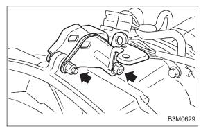
10) Tighten the drain plugs.
