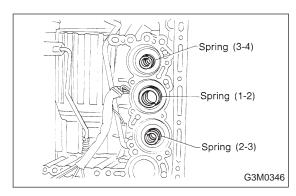
11) Remove the three accumulator springs.
