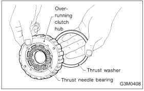
12) Assemble the overrunning clutch hub.
