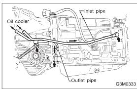
4) Install the oil cooler outlet pipe.
