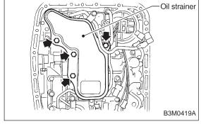
4) Install the oil strainer to the control valve. Be careful not to cut or break the O-ring. Then tighten four bolts.
