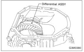
6) Install the differential assembly to the case, paying special attention not to damage the speedometer gears (drive and driven) and the inside of the case (particularly, the differential side retainer contact surface).
