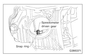
5) Remove the snap ring. Then remove the speedometer driven gear.
