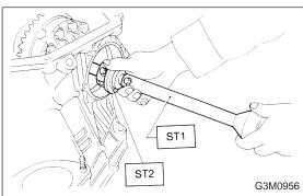
3) Extract the axle shaft with ST1 and ST2.
