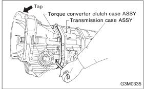
2) Install the torque converter clutch case assembly to the transmission case assembly, and secure with six bolts and four nuts.
