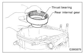
20) Take out the rear internal gear and the thrust bearing.
