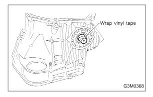
9) Install the oil seal and outer race (taper roller bearing) to the differential side retainer. Then screw in the retainer and the O-ring after coating the threads with oil.
