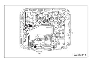
6) Install the oil cooler outlet pipe, and secure with two bolts.
