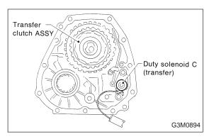
3) Install the transfer clutch assembly to the case.
