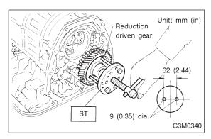
(2) Using the ST, extract the reduction driven gear.ST 899524100 PULLER SET
