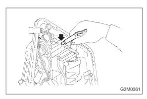
(3) Take out the low & reverse piston by applying compressed air.
