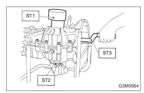
(1) Place the transmission with case left side facing downward and put ST1 on bearing cup.
