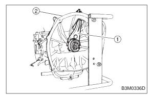
13) Install clutch release lever ① and operating cylinder (hydraulic application type) ②. <Ref. to 2-10 [W3C1], [W3C2], [W5A0].>
