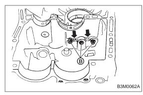
Position interlock plungers (5.56 x 19.6), one plunger in hole between 1-2 and 3-4 fork rod holes, and one plunger in hole between 3-4 and reverse fork rod holes.
