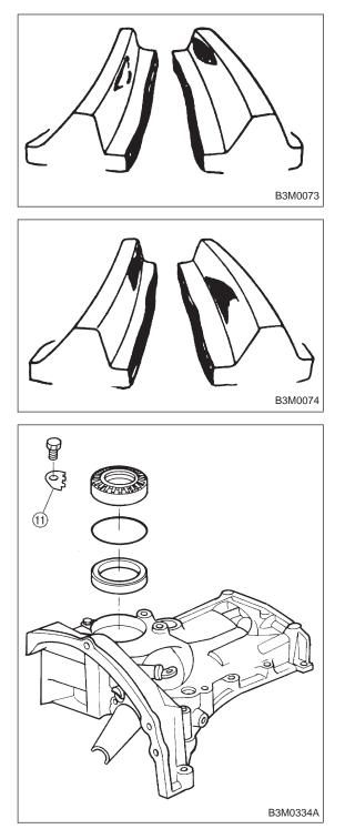
• The drive pinion shim selected before is too thick. Reduce its thickness.
