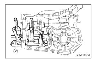
1) Drive out spring pin (1) with ST, and remove 5th shifter fork (2).
