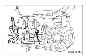
3) Drive out spring pin (6), and pull out 3-4 fork rod (7) and shifter fork (8).
