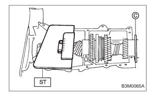
(3) Position the ST by inserting the knock pin of ST into the knock hole in the transmission case.
