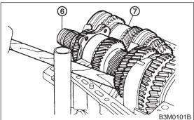
5) Remove drive pinion shaft assembly (6) from left side transmission case.
