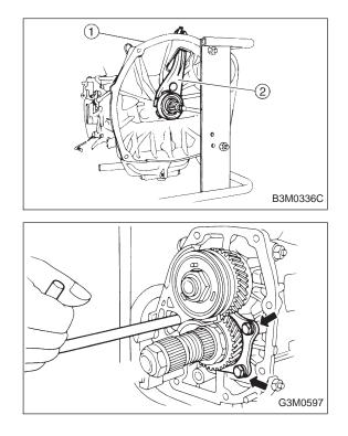
Remove operating cylinder (hydraulic application type)
