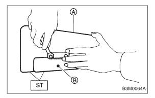
2) Adjustment of drive pinion shim (2)
