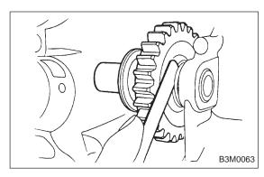
(2) After installing a suitable reverse shifter lever, shift into neutral. Using a thickness gauge, measure clearance between reverse idler gear and transmission case wall and adjust with washer(s).
