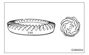
1) Alignment marks/numbers on hypoid gear set ① The upper number on driven pinion is the match number for combining it with hypoid driven gear. The lower number is for shim adjustment. If no lower number is shown, the value is zero. The number on hypoid driven gear indicates a number for combination with drive pinion.
