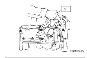
(3) Remove weight and screw in retainer without O-ring on the upper side and stop at the point where slight resistance is felt.
