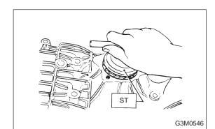
9) Remove outer snap ring (2) and pull out speedometer driven gear (2). Next, remove vehicle speed sensor 2, oil seal, speedometer shaft (2) and washer.
