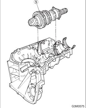
5) Install drive pinion shaft assembly (5) with shims selected before into transmission case.
