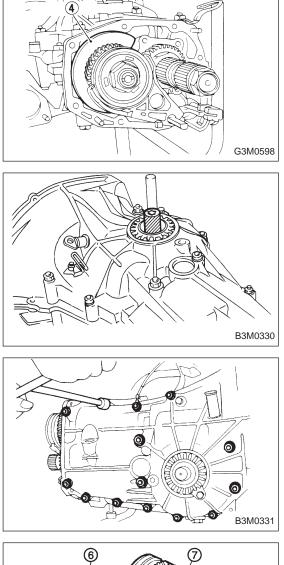
3) Remove main shaft rear plate ④.
