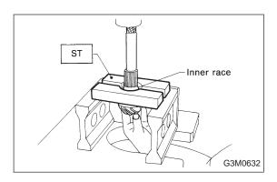
8) Remove 1st gear bushing, 1st driven gear thrust plate, and roller bearing (41 x 71 x 23) using ST and press.
