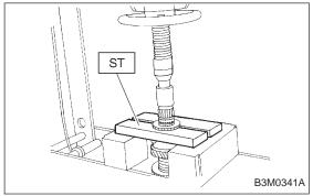
2) Remove 5th driven gear using a press.
