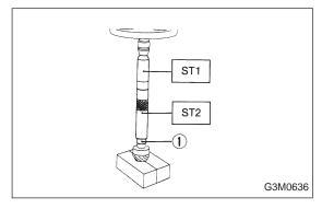
4) Install 1st-2nd driven gear bushing ① onto drive pinion shaft.
