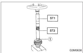
7) Install 1st-2nd driven gear bushing (1) to drive pinion shaft using ST1 and ST2.
