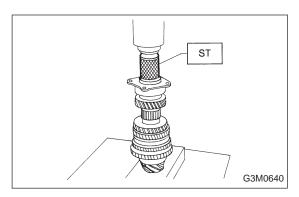
10) Install ball bearing (29 x 74 x 38) on drive pinion shaft with ST.
