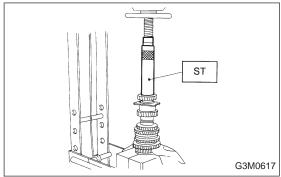
11) Position woodruff key in groove on the rear of drive pinion shaft. Install 5th driven gear onto drive shaft using ST and press.
