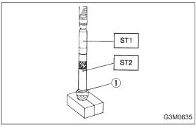
3) Drive roller bearing onto drive pinion shaft and 1st driven gear thrust washer ① using ST1 and ST2.
