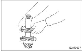
6) Install 1st driven gear, 1st-2nd balk ring and gear and hub assembly (already assembled in previous step) to drive pinion shaft by hand.
