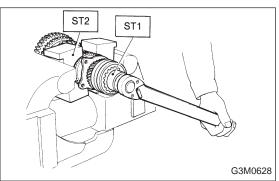
12) Install lock washer and tighten lock nut to the specified torque using ST1 and ST2.
