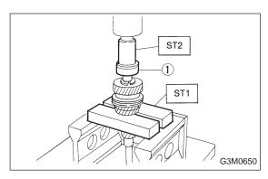
5) Drive ball bearing ① onto the rear section of transmission main shaft using ST1, ST2 and a press.
