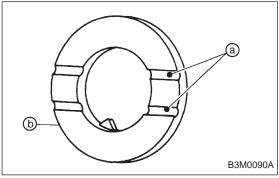
4) Install baulk ring, needle bearing (32 x 30 x 25.7), 4th drive gear and 4th gear thrust washer to transmission main shaft.
