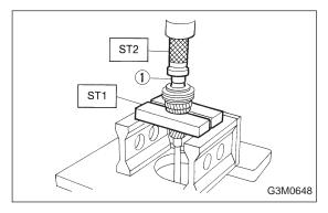
3) Install 4th needle bearing race ① onto transmission main shaft using ST1, ST2 and a press.
