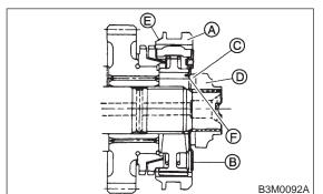
7) Install the following parts to the rear section of transmission main shaft.
