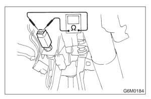
CHECK : Is the resistance less than 10  $\Omega$ ? (With pedal released)
