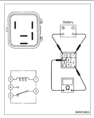
CHECK : Is starter interlock relay normal?
