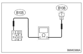
(CHECK): Is the resistance less than 10  $\Omega$ ?
