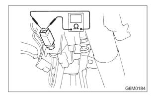
CHECK : Is the resistance more than 1 M $\Omega$ ? (With pedal depressed)
