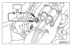
1) Check for open circuit. (range:  $\Omega \times$  1K) Measure the resistance between the respective pins in both connectors.
