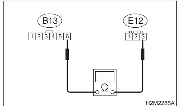
**CHECK** : *Is the resistance less than 1 Ω?*
