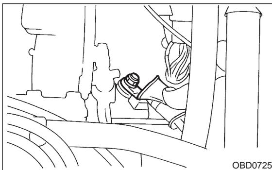
3) Measure resistance of ground cable between ground cable terminal and engine ground.
