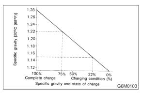
(2) Measuring the specific gravity of the electrolyte in the battery will disclose the state of charge of the battery. The relation between the specific gravity and the state of charge is as shown in figure.
