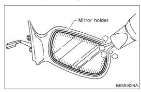
3) Remove mirror plate while lifting the mirror holder using a flat bladed screwdriver.
