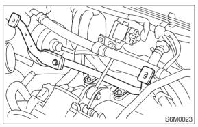
4) Remove bolt which installs hill holder cable bracket. (2200 cc MT model with hill holder)
