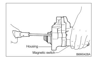
9) Remove housing from magnetic switch.
