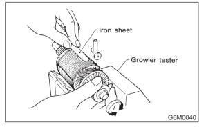
5) Armature ground test
