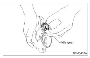
13) Remove retainer and roller from housing.
