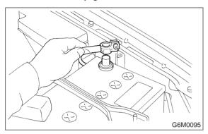
2) Disconnect connector from ignitor.
