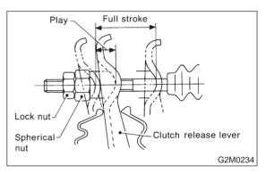
3) Upon completion of adjustment, securely lock spherical nut with lock nut.
