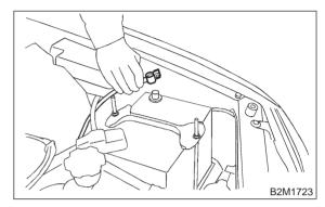
2) Remove air intake chamber and air intake duct as a unit. <Ref. to 2-7 [W18A0].>
