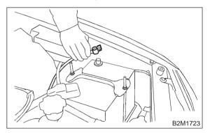
4) Disconnect fuel delivery hose (A), return hose (B) and jet pump hose (C).
